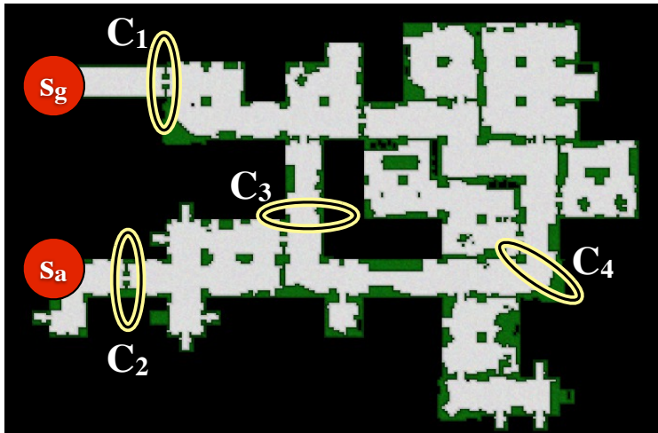
Figure 5: A two-dimensional pathfinding search problem with the goal state labeled s_g and the start state labeled as s_a . C_1 , C_2 , and C_3 \cup C_4 are all cut sets.
