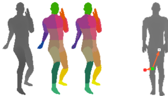
Figure 7: Left: ground truth depth, ground truth body parts and predicted body parts; Right: features specified by offsets u and v .
