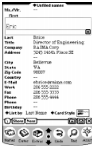
Figure 1: Names application included with all Newton computers depicted at one quarter life size of the Apple Newton MessagePad 100 used in the experiments. As the user taps on a field, it expands to ease writing. In this picture, the First Name field is expanded. The folder tab button at the top of the screen is for displaying names from one of eleven user-defined folders. From left to right, buttons at the bottom of the application screen are for showing the time and battery state (labeled with a clock face), changing the display of this name (labeled “Show”), adding a new name (labeled “New”), refiling this name (labeled with the file folder picture), printing/faxing/infrared beaming/mailing/duplicating/deleting this name (labeled with the envelope picture), and closing the application (labeled with a large “X”). Below these are universal buttons visible in all applications. From left to right, they provide access to the Names application, a calendar application, a storage place for all other applications, scrolling buttons, undo, find, and natural language recognition.
